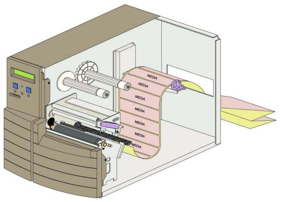
Figure 7-5b, Printer Loading Diagram
